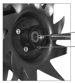
Simply slide the Weed Reducers over the extended part of the tine. The larger part of the Weed Reducer should face transmission.
